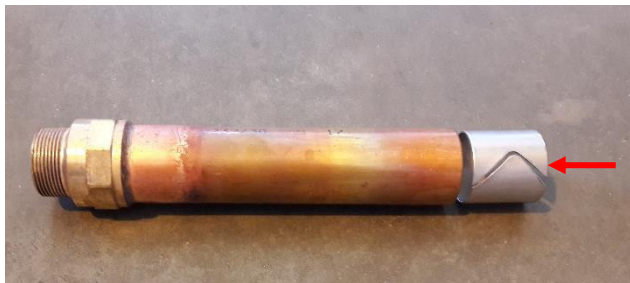
Figure 58: Copper pipe with reinforcing ring
