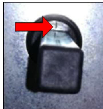
Figure 44: Closed position, characterized by a marking on the gear wheel
