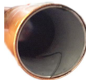
Figure 59: Copper pipe with inserted reinforcing ring
