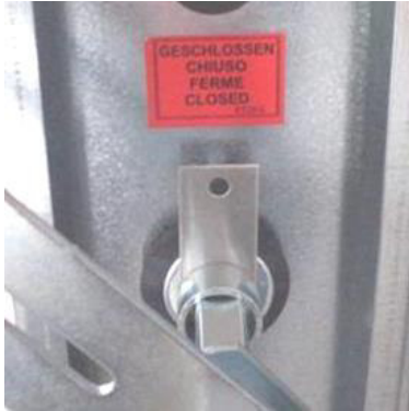
Figure 145: Closed position, characterized by a sheet metal position indicator
