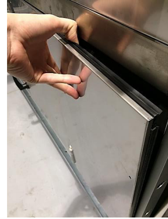
Figure 62: Removal of the external panels
