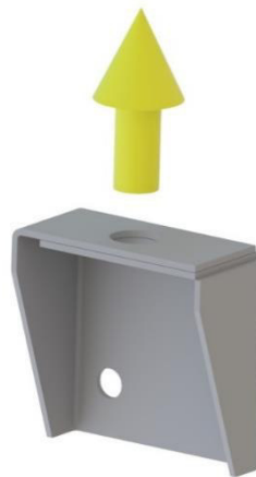
Figure 48: Vertical force transmission on mounting lugs ZHK RECO
