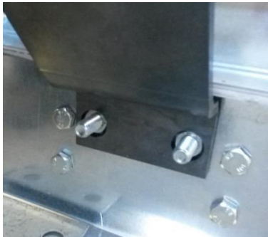
Figure 29: Positioning of the monobloc crane lifting lug at the counter frame
