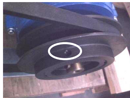
Figure 229: Position of the Allen screws on variable pulleys
