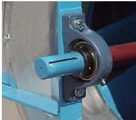
Figure 231: Fan bearing with grease nipple (example Comefri NTHZ)
