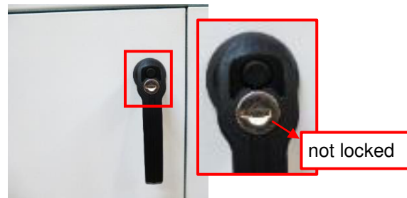
Figure 119: Door ,closed', not ,locked'
