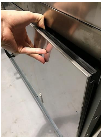
Figure 96: Insertion of the outer panel
