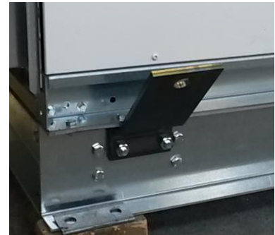
Figure 31: Monobloc crane lifting lugs mounted
