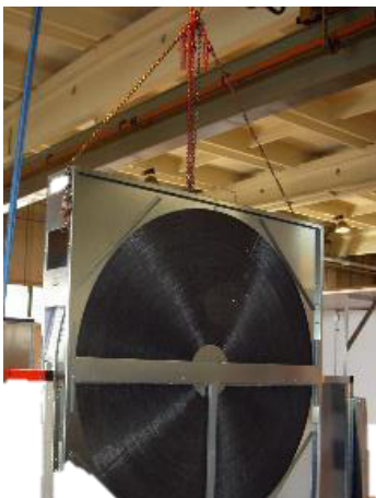
Figure 247: Lifting with chain hoist
