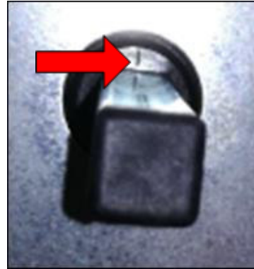
Figure 146: Closed position, characterized by a marking on the gear wheel
