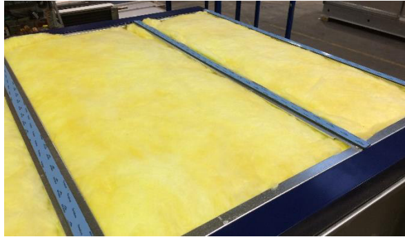
Figure 107: Part of the AHU prepared for assembly of metal sheet roof
