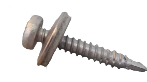
Figure 108: Drilling screw countersunk head TORX 25 with sealing ring \varnothing 4,8 x 30
