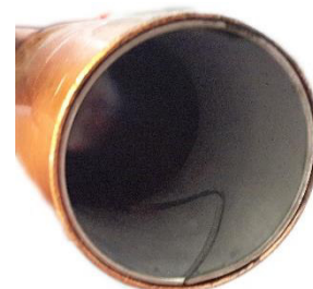
Figure 177: Copper pipe with inserted reinforcing ring
