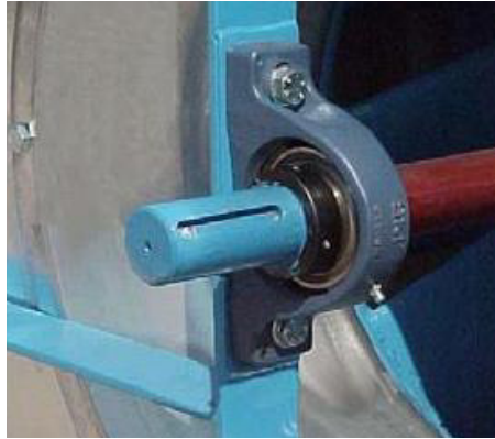
Ilustrație 219: Fan bearing with grease nipple (example Comefri NTHZ)
